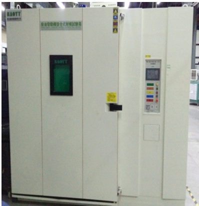
复合式耐候试验箱 Temperature+Humidity+Pressure+Solar radiation composite diesel environment chamber
